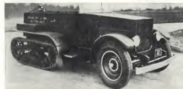
Top: The Half-Track Car T1E1. Above: Half-Track T1. Both were American-built derivations of the French Citroen-Kegresse and represented the first steps into the American half-track field. All pictures courtesy Col R. J. Icks and R. M. Hunnicutt.
